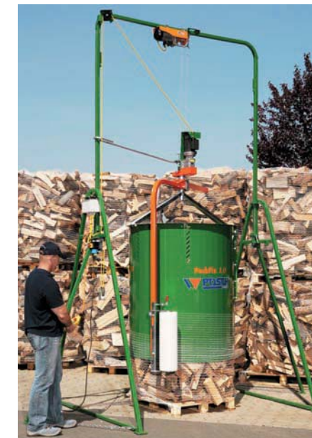
The rotating arm wraps the drum with the net.
