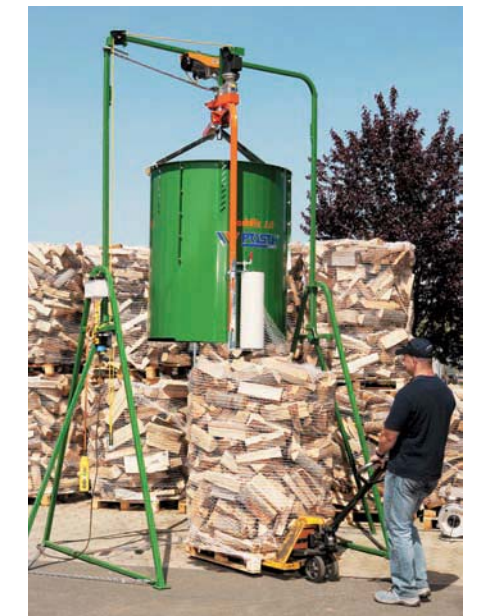
After the drum has been pulled up high enough, the finished pack of timber can be moved away.
