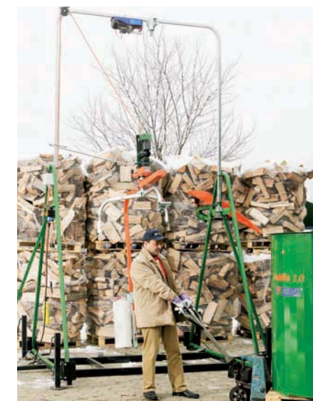
PackFix with “quick-change” system: The full drum is transported to the frame where the net is wrapped around it. (F0002548 base frame with feet as accessory part).
