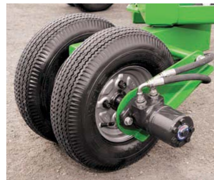
SH: The hydraulic drive allows tilting of the conveyor belt by up to +/-90°.
