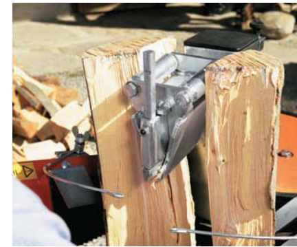
Push-on knife with rollers (F0002544, standard for Special models of log splitters)
