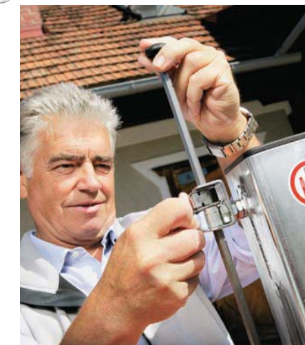
Adjust the splitting stroke with a flick of your hand
