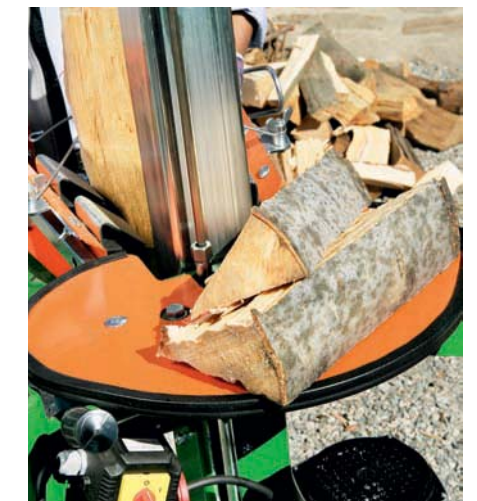
During splitting, billets can be placed on the timber support table.
