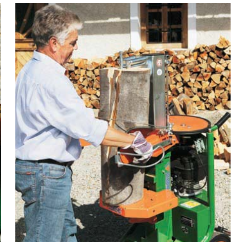
The push-on splitting knife with rollers helps to split even tough wood without any problems.
