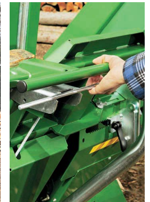
CutMaster 700 Comfort with hydraulically controlled tilting unit
