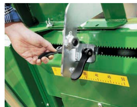
The mechanic stop for infinitely variable adjustment of cut-off length is easy to operate
