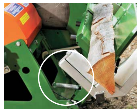
CutMaster 700 Compact, with spring-supported rocker.
