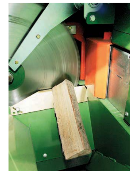
The automatic timber holder ensures safe cutting
