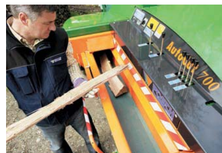
Simple and safe advance of timber via the feeder trough
