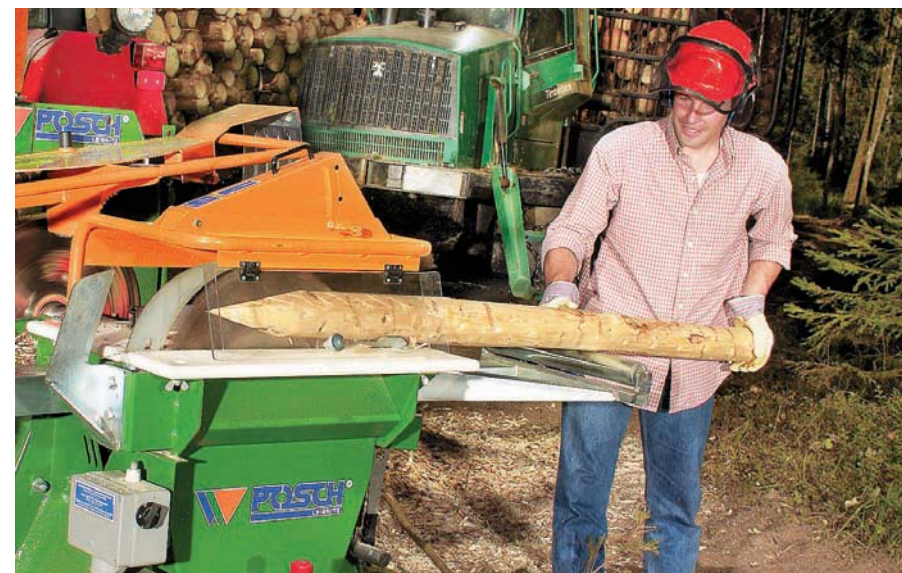
Schälprofi 500 with circular saw attached
