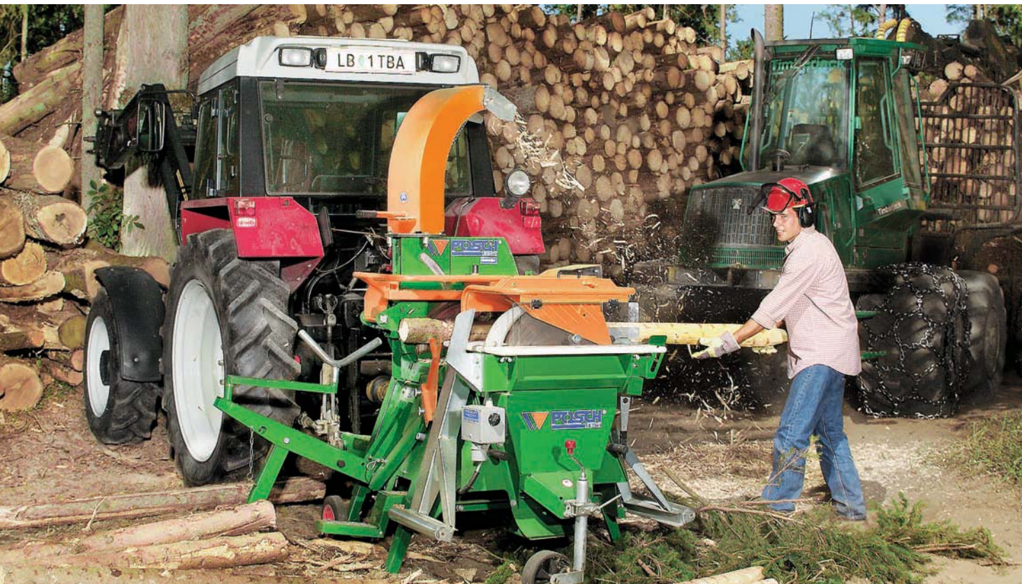
Schälprofi 500 with circular saw attached and combined drive (electric motor and power take-off shaft)
