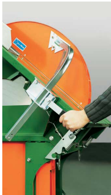
Height adjustable protective cover; no tools needed for adjustment.
