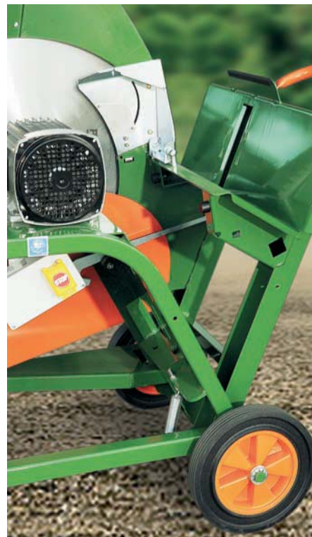
Extremely smooth tilting with enhanced damping mechanism; height-adjustable handle for ease of operation. Large solid rubber wheels, Ø 300 mm, for transportation.
