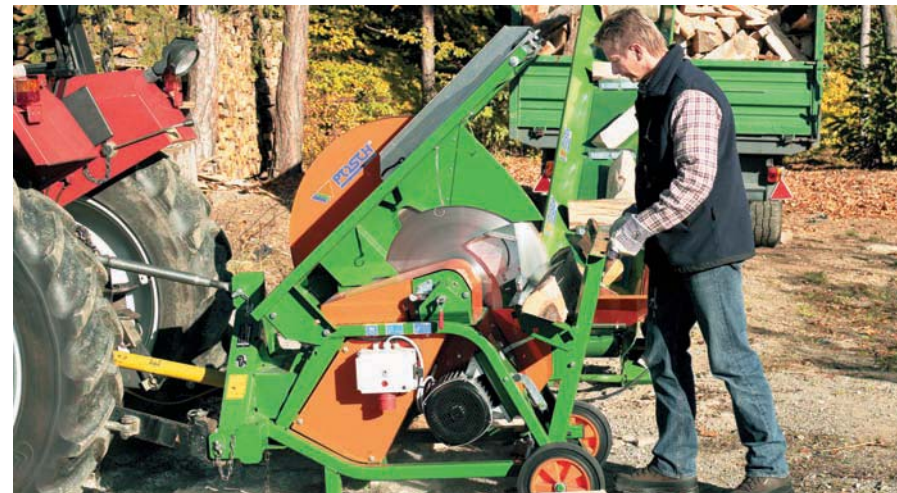
A combination of pto drive and electric motor for flexible application.
