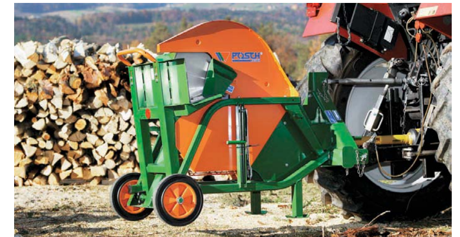
Tilting saw with pto drive. Easy to transport thanks to three-point linkage
