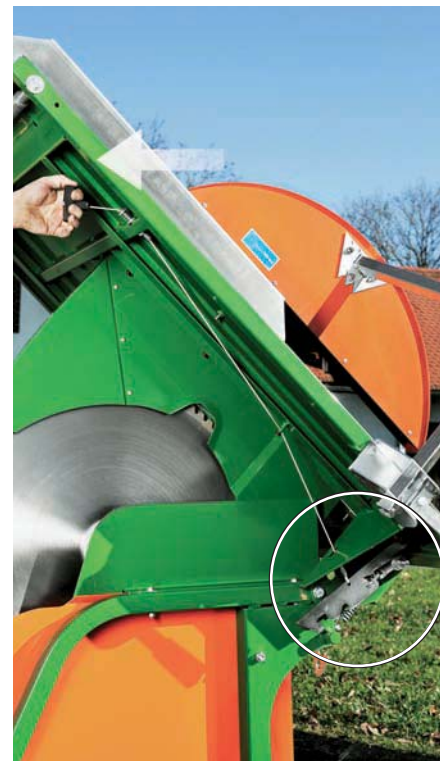
New, convenient mechanism for unlocking the table to change from table to tilting position
