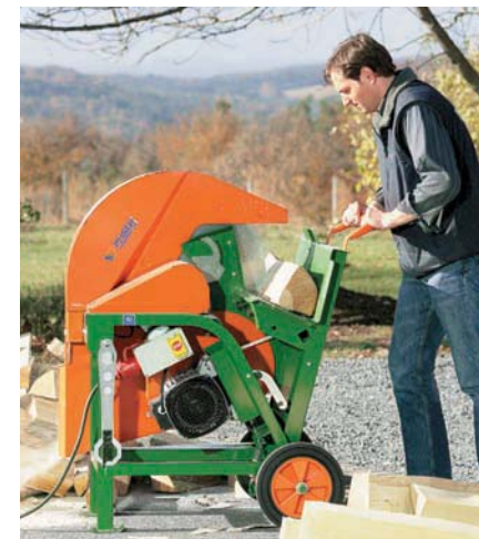
Tilting saw with V-belt drive for powerful cutting of firewood
